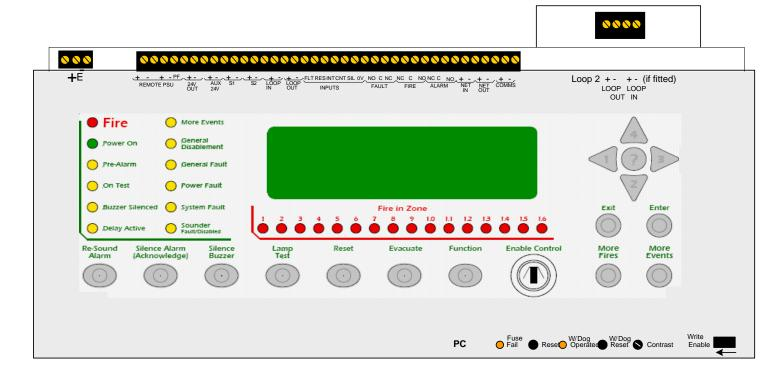
With the lid of the control open, more controls are revealed. These controls are strictly for service personnel and should not be operated by the user under any circumstances. Opening the front cover also gives access to the PC connection port for programming.
