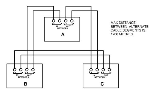
Network boards are fitted with isolators, which disconnect faulty sections of cable and allow the network to continue working by using the return path so it is most important that this wiring configuration be adhered to.
