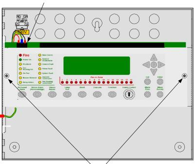
power terminal block from the left hand side of the circuit board, remove the two screws holding the plate in position and then remove the complete circuit board and plate.
