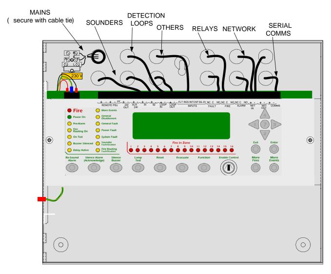
To avoid the possibility of a confusing array of fault conditions, it is best to connect the system gradually so that faults can be cleared on one circuit before connecting another.
