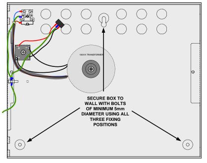
Remove knockouts from the top and or back of the box in the positions at which cables will enter.
